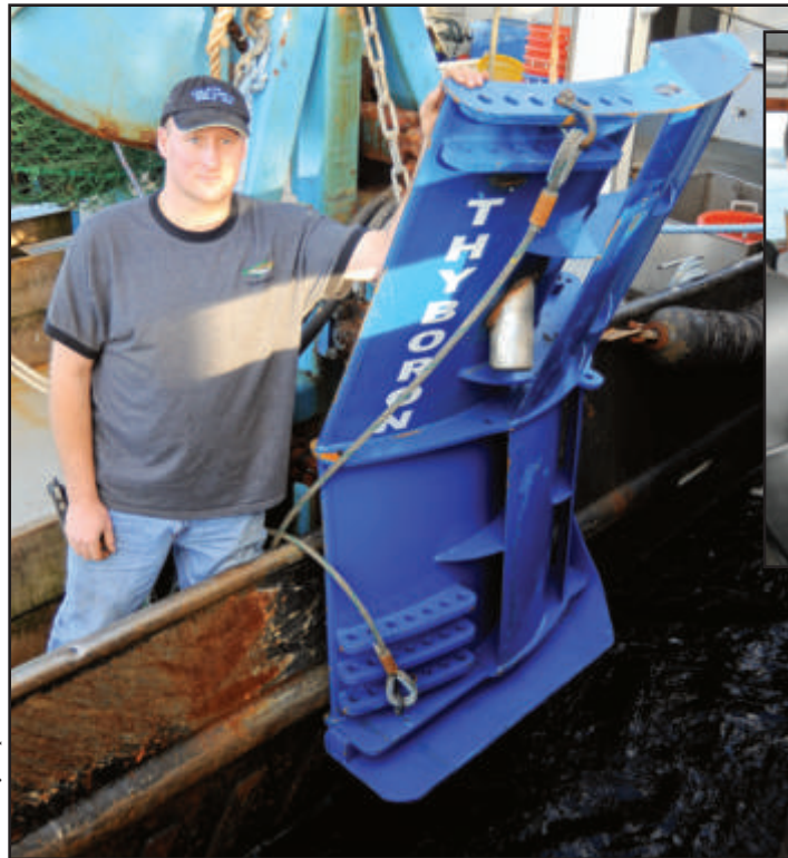
Capt. Jim Ford alongside one of the pair of Thyboron Type 14 semi-pelagic trawl doors that he now fishes. The Danish-made doors are supplied by Trawlworks Inc. of Narragansett, RI.
